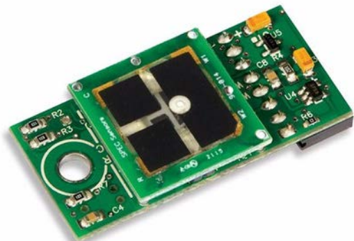
Fig.1. General view of the sensor DGS-NO 2 968-037
