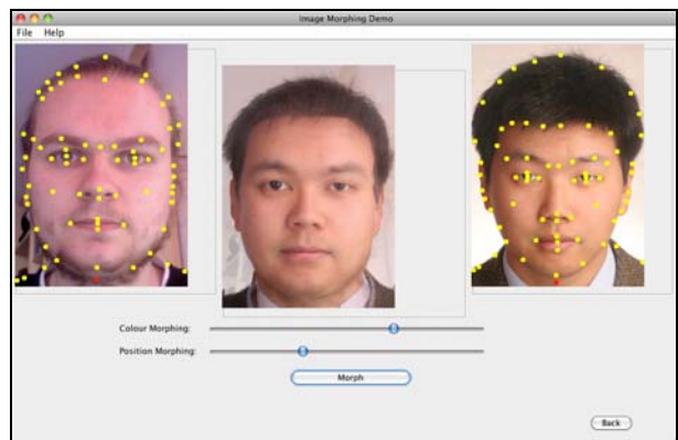
Fig. 13 – Final image from manual determination of reference points by a male user
