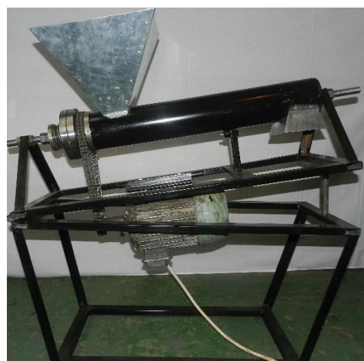
Fig. 4 – Bench for research of reciprocating screw conveyer with flexible working part
