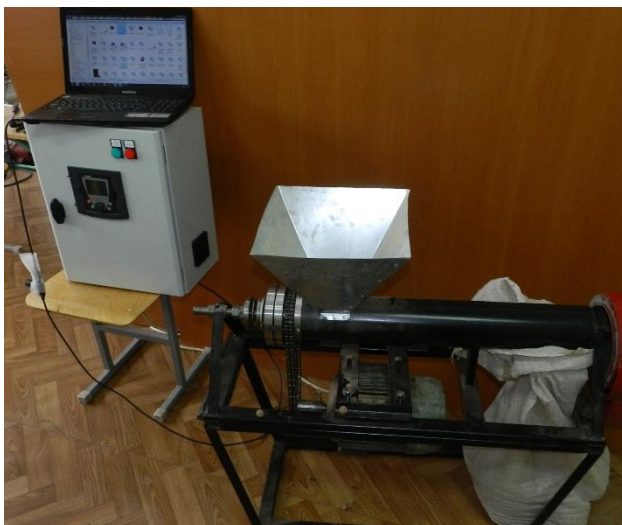
Fig. 4 – Bench for research of reciprocating screw conveyer with flexible working part
