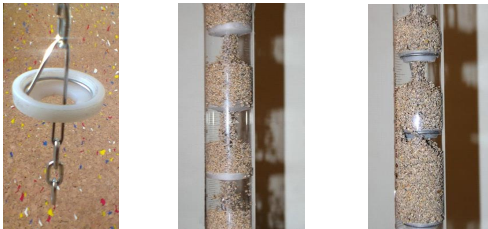
Fig. 4 - A beaded operating element and the process of transporting and stirring of mixed fodder in a vertical route segment of a technological lane
