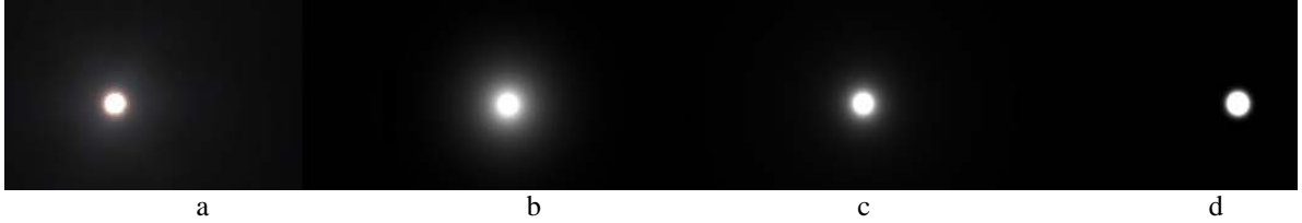
Fig. 5. Demonstration of highlights: a – measured data from chrome sample, b – proposed model, c – Trowbridge-Reitz model, d – Beckmann model [3]
