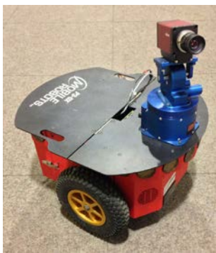
Fig.5. One video-camera application for navigation of mobile robot Pioneer P3-DX (potential application) [21]
