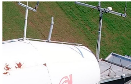
Figure 3. An example of an image for a wind turbine with corrosion [45].
