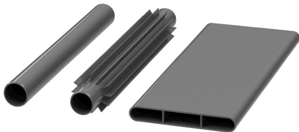
Figure 8. Different shapes of heat transfer surfaces made of polymer composites with enhanced thermal conductivity [76].
