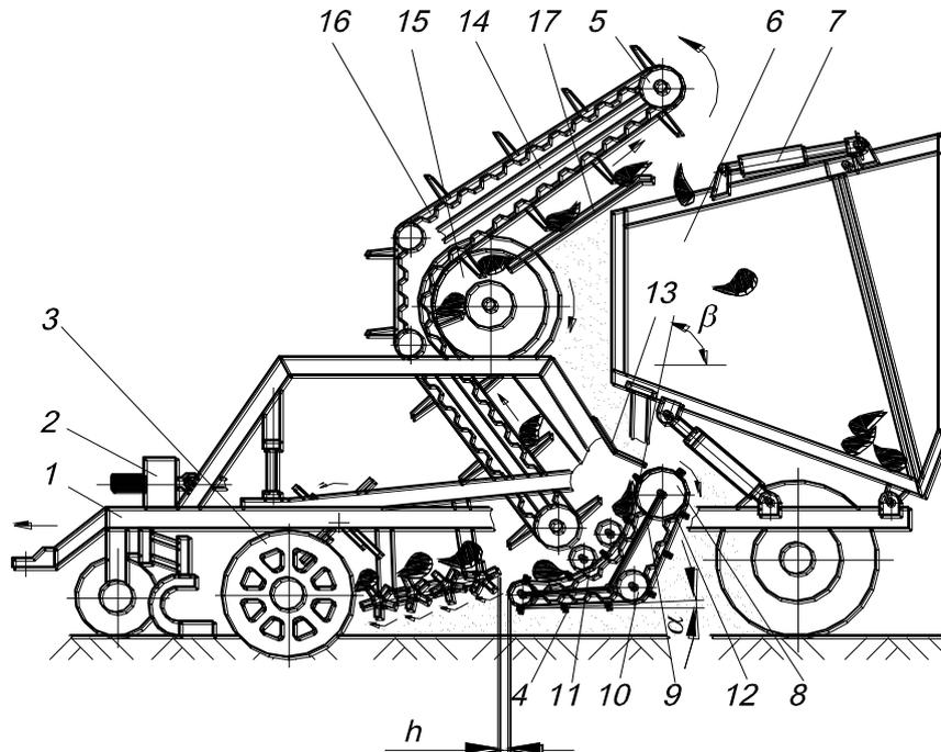
**Fig.3 – Design and process flow sheet of a semi-trailing root crop harvester**
