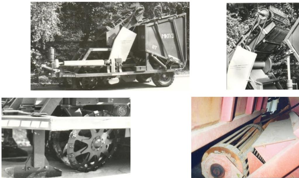
Fig.5 – Overall view of a root crop harvester and its operating elements
