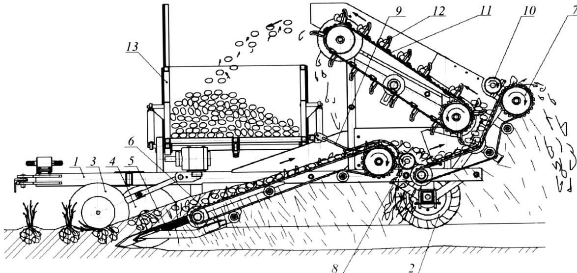
**Fig.2 – Design and process flow sheet of a potato harvesting machine**
