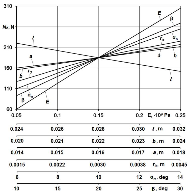
**Figure 4.** Graphical dependencies for the evaluation of intensity impact of interworking parameters of auger operating surface and corn grain on the value of circular force  $N_o$
