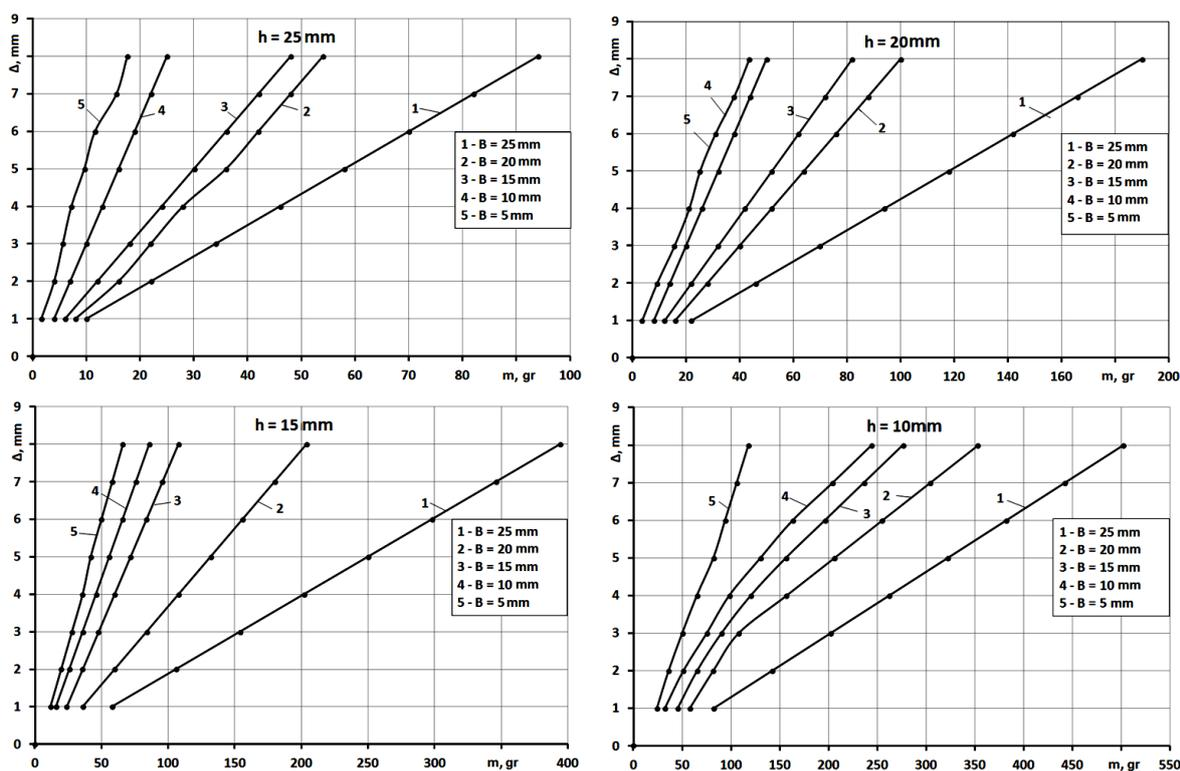
**Figure 7.** Experimental research findings for the dependency of blade running end deformation value  $\Delta$  from measured load mass  $m$  for different values of  $B$  and  $h$
