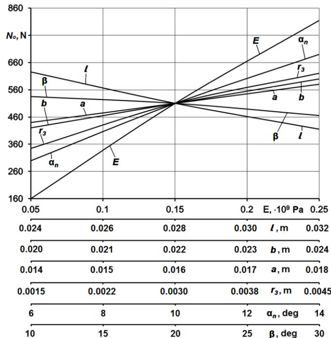
**Figure 3.** Graphical dependencies for the evaluation of intensity impact of interworking parameters of auger operating surface and corn grain on the value of axial force  $N_o$
